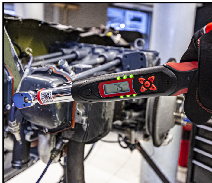
EDWS030 tighten bolts on a engine.
